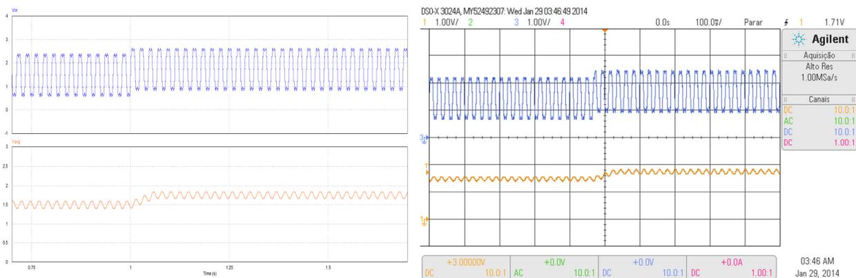
Fig. 9: Input (blue) and Output signal for N=54 (orange).
